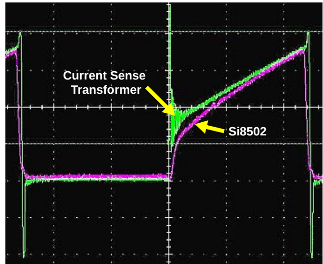
Figure 8. Leading-Edge Noise Suppression Waveforms (200 kHz, 9.3 A Load)
